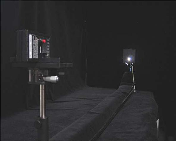
Fig. 1.— Measurement of the acceptance angle.
