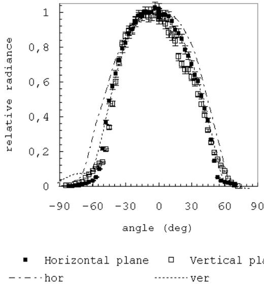
Fig. 3.— Angular response of SQM in a linear scale. Lines show the normalized output frequency of the detector at each angle provided by the detector manufacturer, along the vertical (dashed) and horizontal (dot-dashed) planes.
