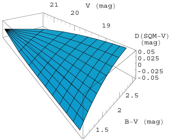
Fig. 20.— SQM-V conversion factor (mag arcsec<sup>-2</sup>) for a night sky model spectrum, in function of its V brightness and B-V color index.
