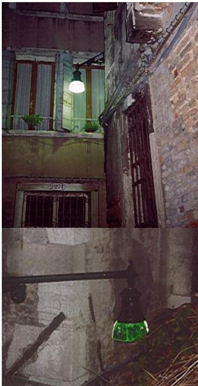
Figure: Top: A luminaire strongly illuminates directly inside a house. Bottom: A home-made but functional screening has been obtained by the city technicians varnishing with dark paint a section of the glass of the fixture.
